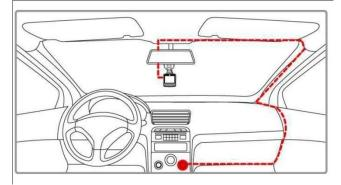
1. Connect one end of the car charger to the USB connector of the camcorder. *USB port input: DC 5V / 1A.*
