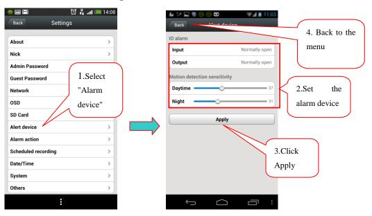
I / O Alarm input: Connect the camera alarm input to the alarm sensor (like Door contact, infrared, smoke detector etc.), make sure the alarm sensor are normally-on, when alarm event occurred, alarm device switch off and trigger a camera with the arming.
