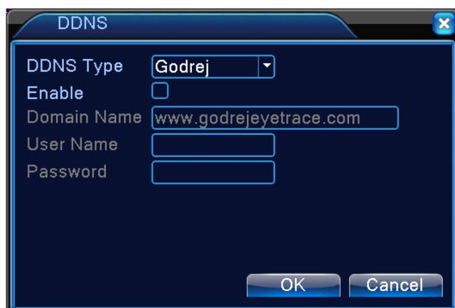
**【DDNS】** User can set up the DDNS and remotely access the DVR via DDNS on browsers.
