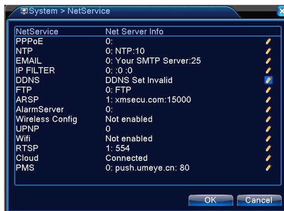
**【PPPoE】** User can directly connect the DVR to internet via ADSL, then input the user name and password;
