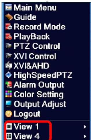
Depending on the DVR model (4-Channel / 8-Channel) you bought, you will have different options on the view mode. There is single-cam view, quad-cam view, multiple camera view, etc.
