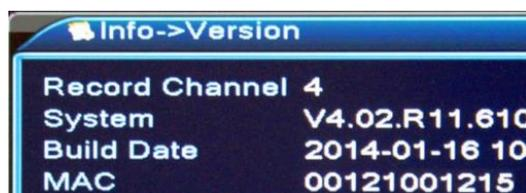
Step 3: Using a web browser, go to <http://xmsecu.com:8080> and login using the MAC number. If it fails to login, verify the MAC number, and try logging in again. Current information about the DVR will be shown. "True IP" is the current external IP address of the DVR.
