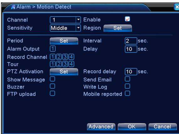
**【Channel】** Choose the channel camera to detect movements.
