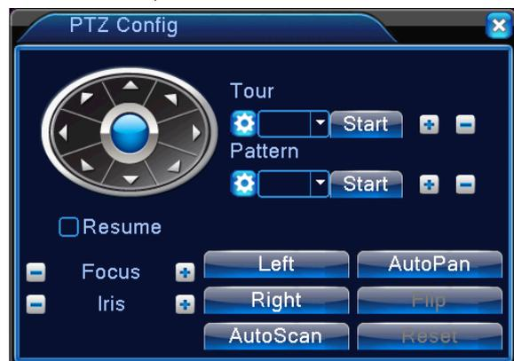
【Tour】 In Tour, you can move the PTZ to different key points and make it stay there for a defined duration before moving on to the next point. The key points are defined by presets. You will need to set all the preset positions before you use the Tour function.
