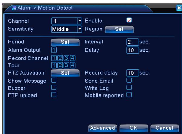
**【Record Delay】** When the alarm is off, the alarm recording normally stops, however, if you set the Delay, the alarm recording will not stop immediately after the alarm is off, instead, it will last a few more seconds/minutes, from 10-300s.
